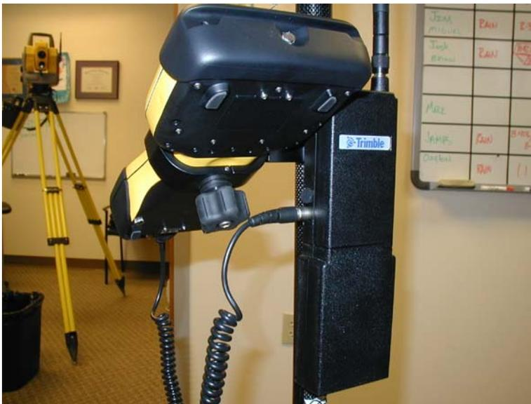
**Note: Attach the controller cable to the bottom port on the radio.**
