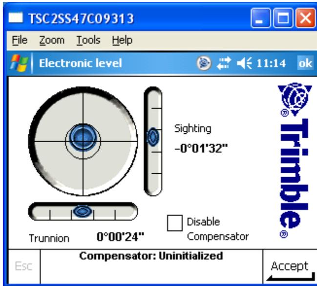
5. Use the electronic level to fine level the instrument. Align the instrument with 2 screws on the tribrach and level the trunnion. Use the third screw on the tribrach for leveling the sighting. Level the instrument to within acceptable survey tolerances.
