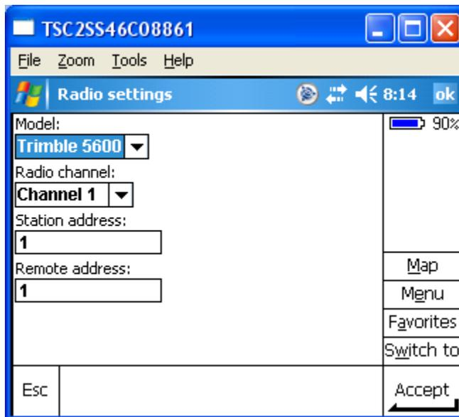
4. Verify the model is 5600, the Radio channel is 1, Station address is 1 and Remote address is one.
