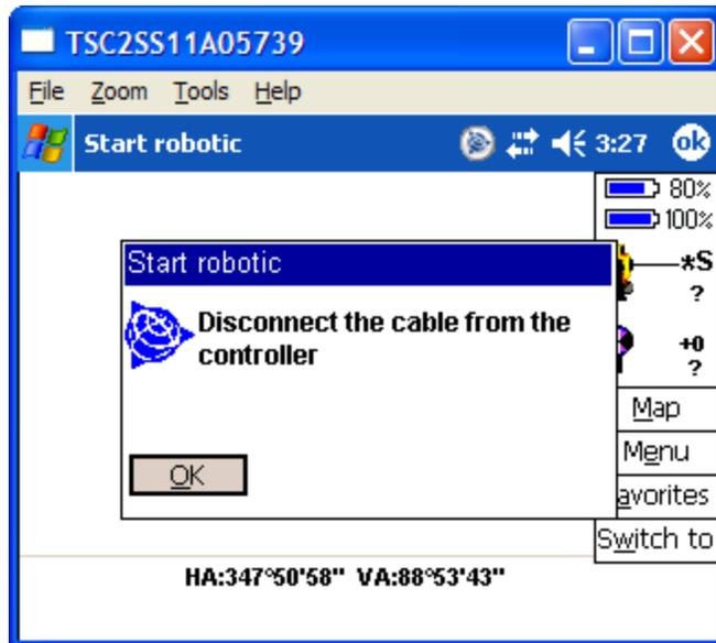
Disconnect the cable from the instrument before tapping on OK.
