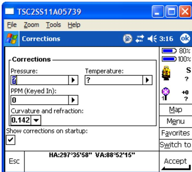
8. Enter the Pressure and Temperature and tap on Accept.
