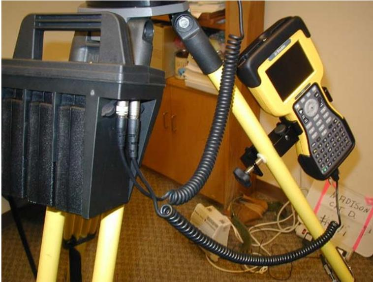
**Note: The data collector cable must be attached to the same side of the battery pack as the power cable.**
