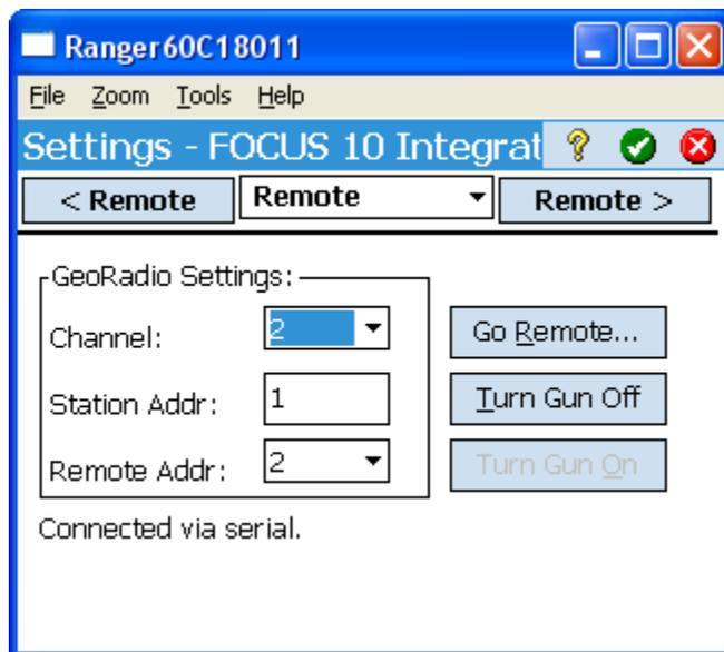
14. Tap on Go Remote. This will put the Focus into Robotic mode and set the Channel, Station Addr and Remote Addr in the instrument.
