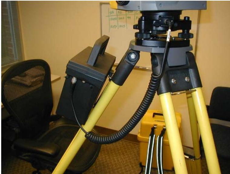
2. Connect the data collector to the battery pack.
