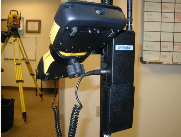
**Note: Attach the controller cable to the bottom port on the radio.**
