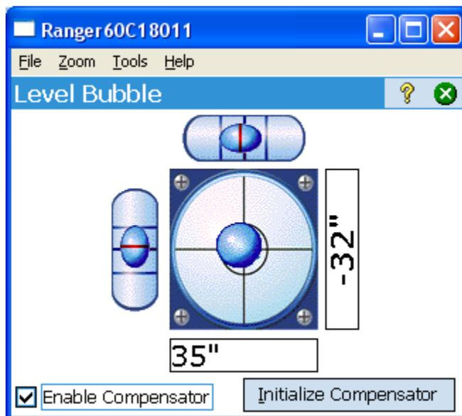
6. Use the electronic level to fine level the instrument. Align the instrument with 2 screws on the tribrach and level the trunnion. Use the third screw on the tribrach for leveling the sighting. Level the instrument to within acceptable survey tolerances.
