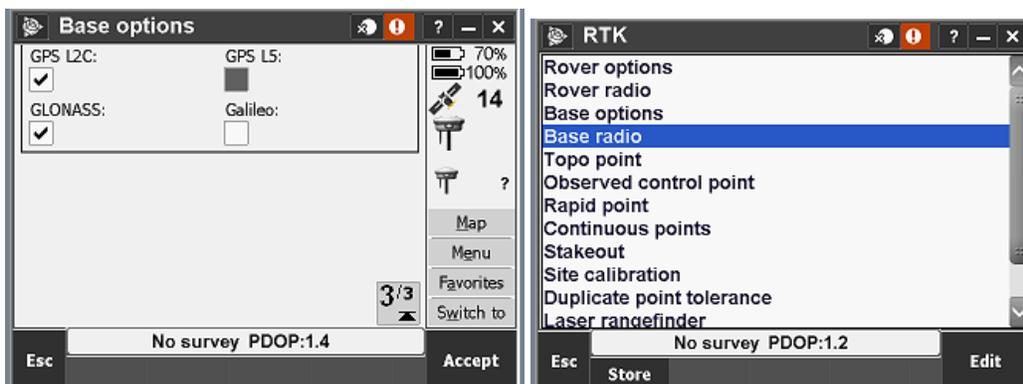
13. Double check the Receiver Port, and make sure what Port the Radio is plugged into on the Receiver. Change the Baud Rate from 9600 to 38400 and click Connect.
